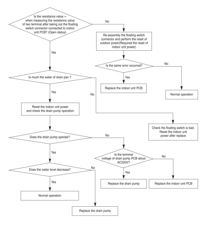
Note: E3 error should be released when indoor unit power is reset.
